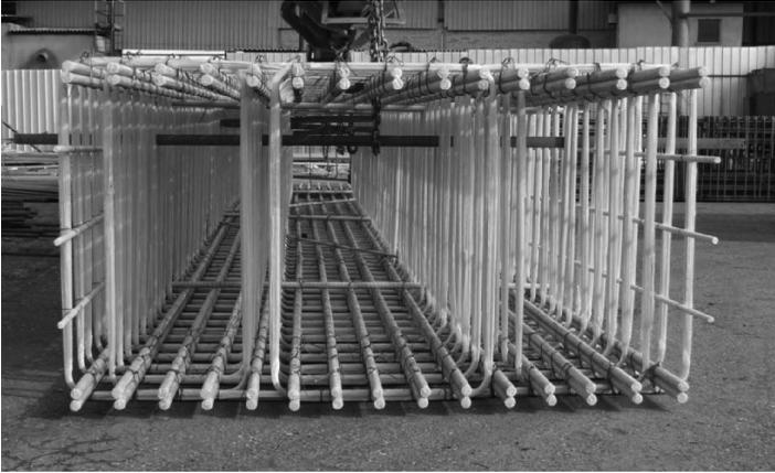
Figure 1.12 GFRP reinforcement cage for soft-eye construction at a manufacturing plant (Angri, Italy).
