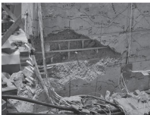
(b) Concrete crushing causing failure
