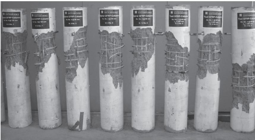
(c) Column specimens after failure
