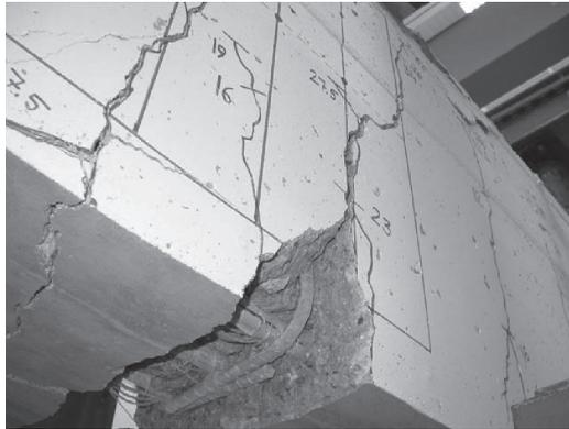
(b) Detail of failed concrete in compression and GFRP bar in tension
