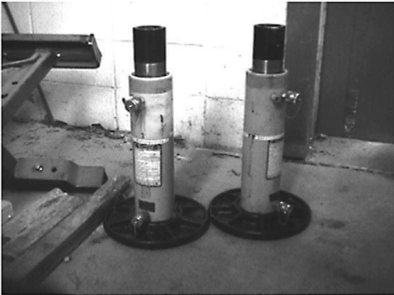
Figure 9.14 Hydraulic jacks used to apply load.
