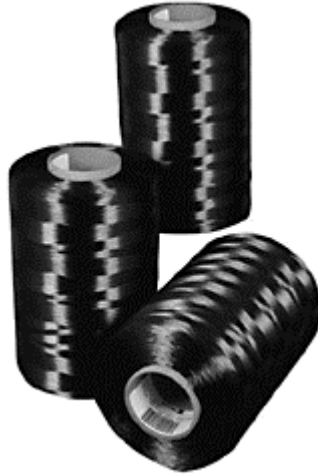
Figure 2.4 Carbon tow wound around spools (Source: Zoltek, 2008).
